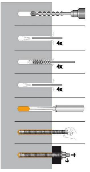
Drill hole of diameter  $(d_0)$  and depth  $(h_0)$  with a hammer drill set in rotation-hammer mode using an appropriately carbide drill bit.
